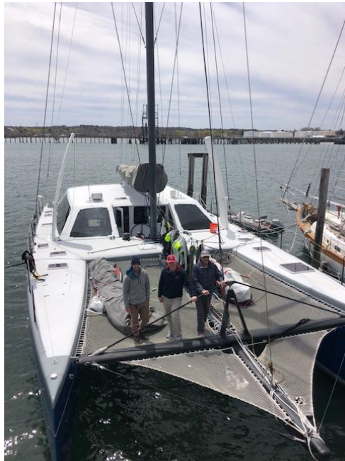
GAIA with captain Andrew Reiley, and delivery crew Toby Reiley and Seamus Hourihan on the bow in Portland, ME. The boat is about the size of a tennis court. The mast is over 100' tall and the dagger boards draw 16' when down.
