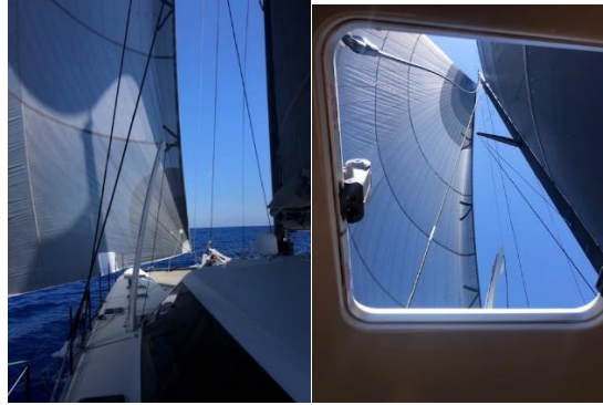
The A3 roller furling headsail. From the deck and as seen through a hatch from below.
