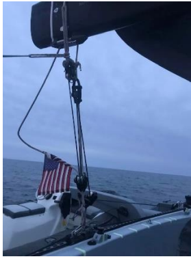
The block and tackle Seamus and Andrew constructed to control the for the rest of the trip. The 16 foot "dinghy" is hanging on the davits behind the traveler.
